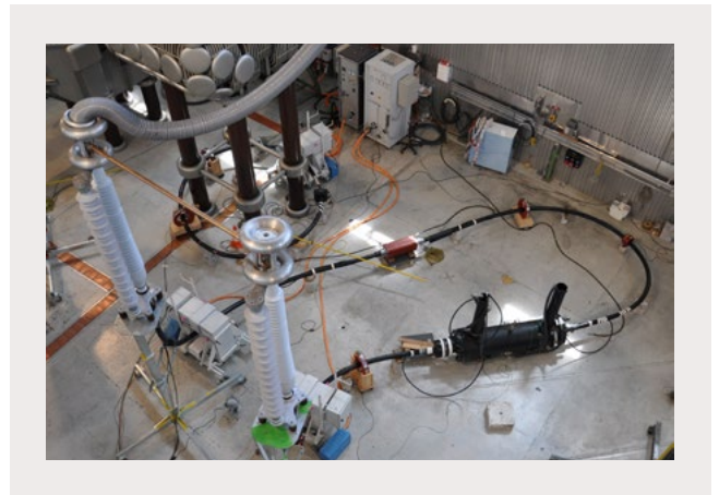
Fig. 11: Setup for the electrical test of the dry type back-to-back joint
