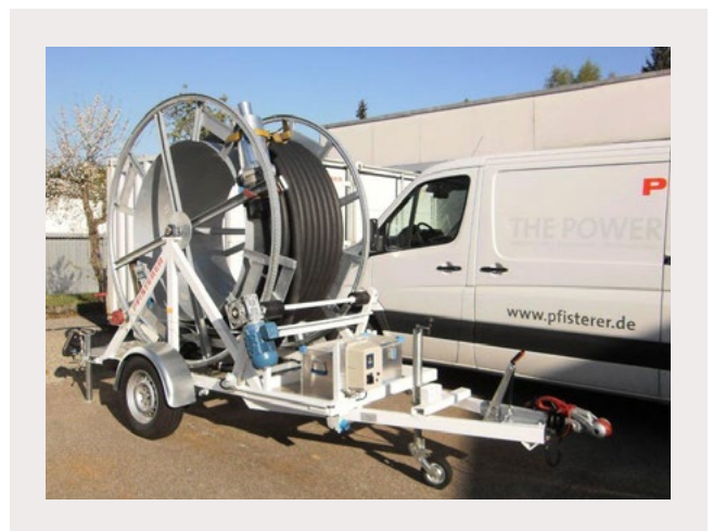
Fig. 17: Cable link on trailer for temporary installation
